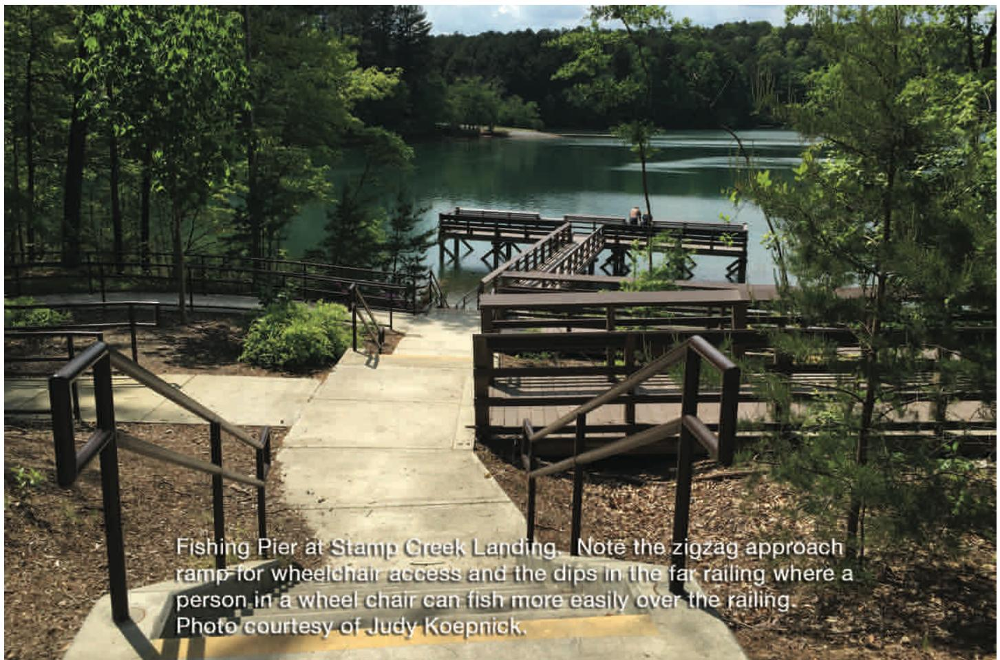
Fishing Pier at Stamp Creek Landing. Note the zigzag approach ramp for wheelchair access and the dips in the far railing where a person in a wheel chair can fish more easily over the railing. Photo courtesy of Judy Koepnick.
